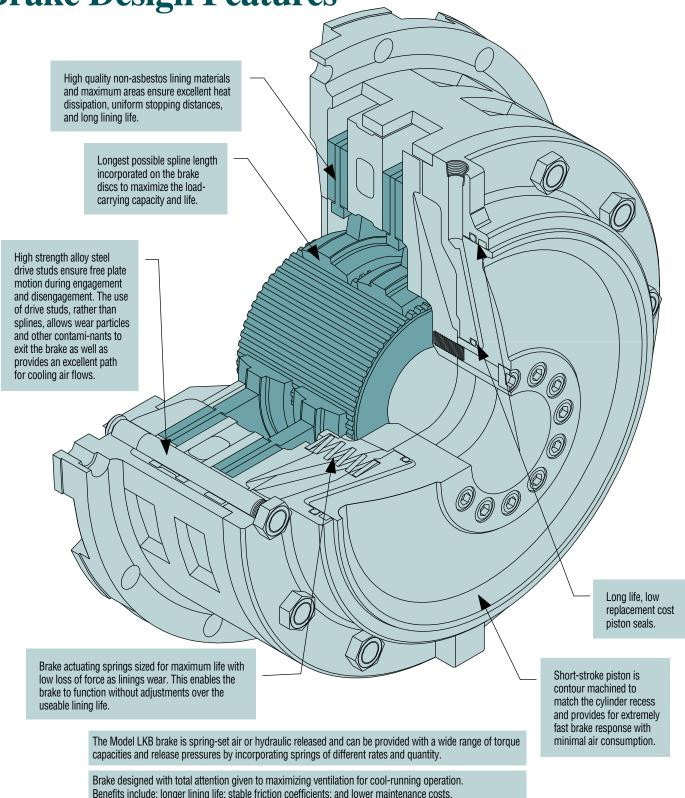
All materials selected and field proven to provide the best available resistance to wear and thermal distress.
