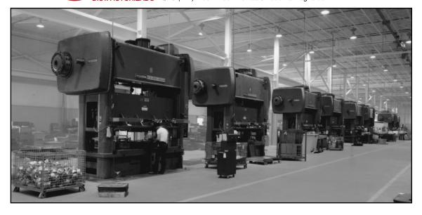
Model LKB-221 **Brakes** installed on a series of 250-ton presses
